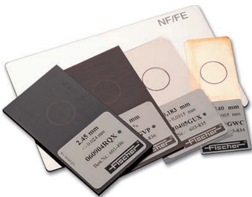
Example of a calibration foil set
