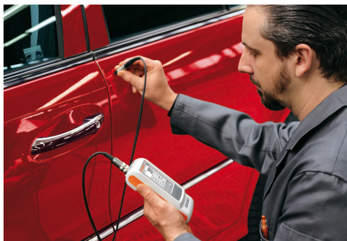
Measurement of car body paint thickness using the dual probe FD10.
