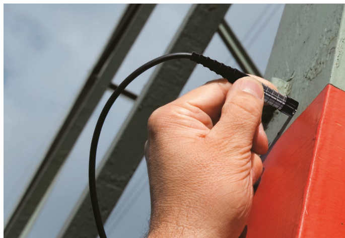
Duplex measurement of paint-zinc coatings with the probe FDX13H.
